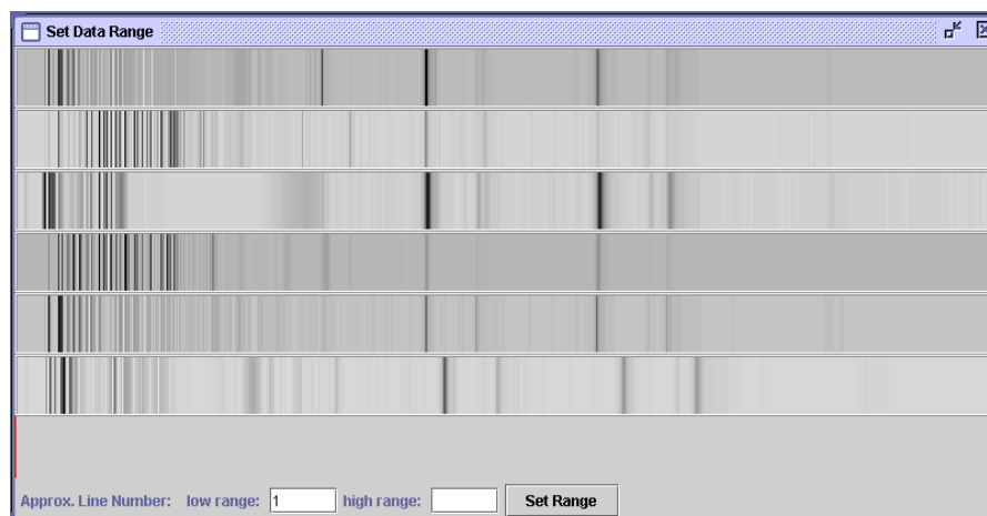
Figure 3-32. Watch out for unusual density plots. Notice how the higher range bands in the bottom plot are displaced from those above. Reexamine how displaced spectra were obtained.
